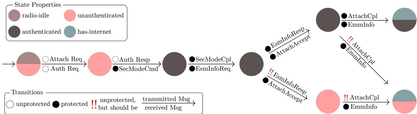
**Figure 5: Path to Internet access for Open5GS. The upper path goes through authenticated states exclusively (correct), however, it accepts unauthenticated messages (lower path) after the Security Mode procedure.**
